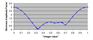
Figure 5. Waviness factor vs. fractional portion of ratio Wheel-RPM/Workpiece-RPM.
