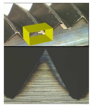
Figure 2. Oxidation burn from thread grinding.
