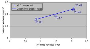
Figure 6. Measured waviness value vs. predicted waviness factor in cylindrical grinding using crude model.
